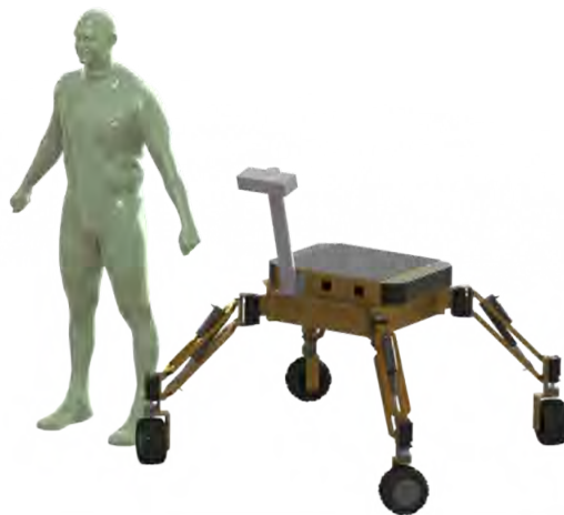
Fig. 1: The MAMMOTH (Mars Analogue Multi-MODE Traverse Hybrid) Rover. The rover is shown next to a 1.8 m tall human figure for scale.
