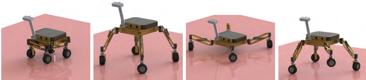
(a) Compact configuration. (b) Tallest configuration. (c) Shortest configuration. (d) Kineo-static walking.
