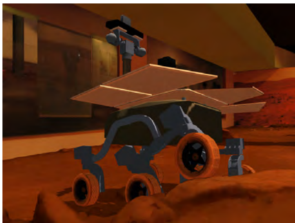
(b) The left bogie tilts without affecting the overall tilting of the body
