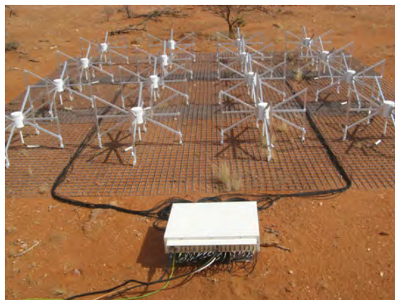
Figure 1: A tile of the Murchison Widefield Array radio telescope, consisting of 16 crossed dipole antennas.
